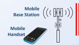
Base station and handset signals easily block the SMATV/TVRO front-end receivers and affect their operation
